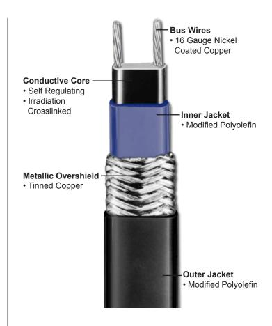
**Applications** for the HTS-6 Self-Regulating Heating Cable:
