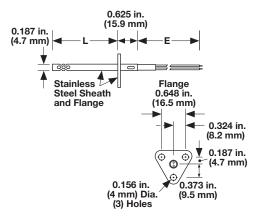
Aspirated tube design allows air to flow directly over thermistor for fast time response with a flange for mounting sensor
