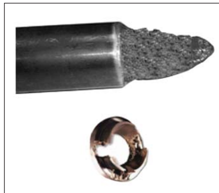
Figure 4: Cavitation damaged valve plug and orifice. Photo Courtesy: Jon Monsen
